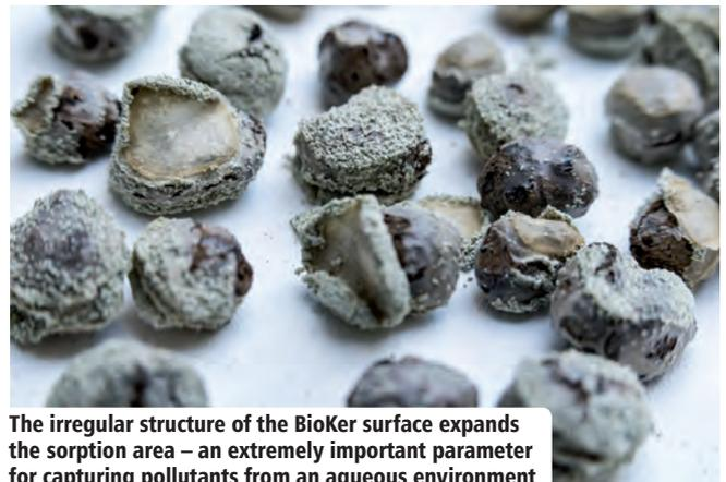
**The irregular structure of the BioKer surface expands the sorption area – an extremely important parameter for capturing pollutants from an aqueous environment**
