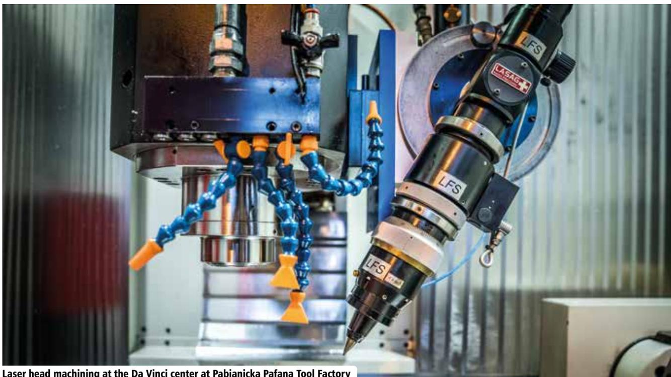
Laser head machining at the Da Vinci center at Pabianicka Pafana Tool Factory
